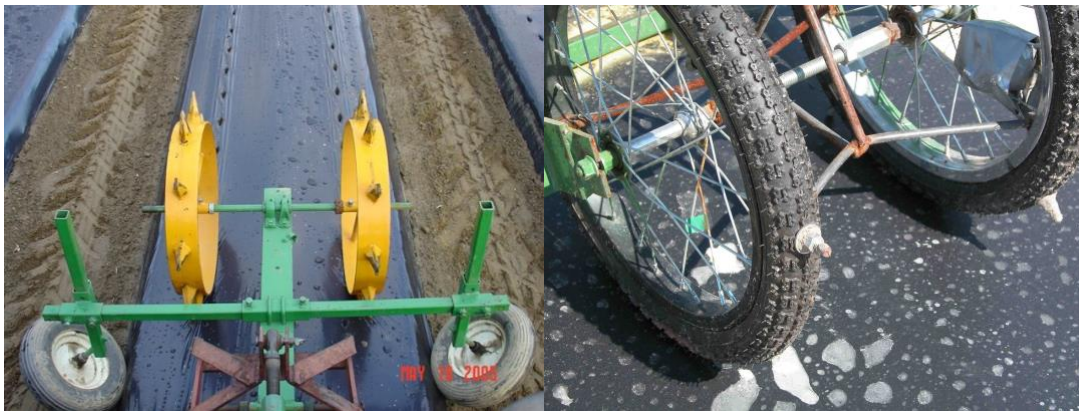
Fig. 7-3. Planting devices: A. Spacing wheel (left). B. Bicycle wheel.
