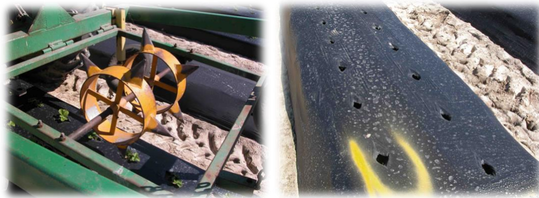
Fig. 7-5. Planting wheel cuts: A. Some planting wheels (left) leave very large cuts in the plastic. B. Large holes in the plastic provide entry for weed seeds, and branch crowns may get caught under the plastic as well.
